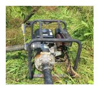
Generator and Sump Pump - Similar to the gas-powered pump system, the generator and sump pump system has the advantage of using a generator that can be multi purpose. A one-way check valve may be required to prevent backflow.
